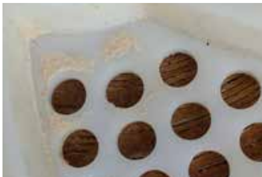
Scaling Particle Pollution on the feed water end-surface of membrane element
