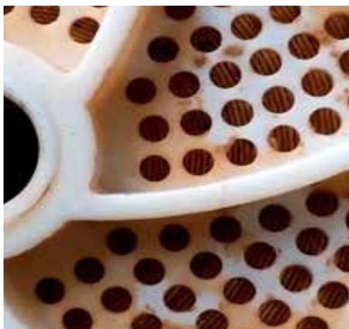
Contamination in feed water end-surface of membrane element
