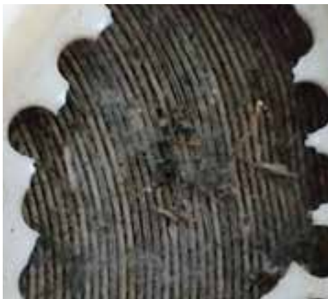
Contamination in feed water end-surface of membrane element
