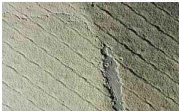
Fouling of membrane sheet surface
