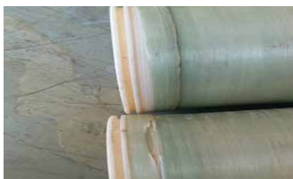
Damage caused by high pressure difference
