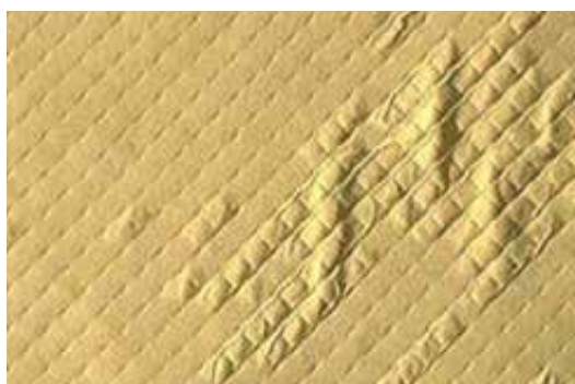
Damage of filter layer caused by back pressure
